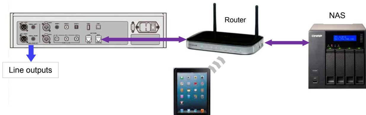
Figure 3 – Using a **Bartók DAC** with a NAS
