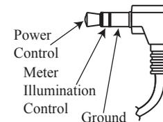
Figure 10– Mini plug for Power Control (Trigger)
