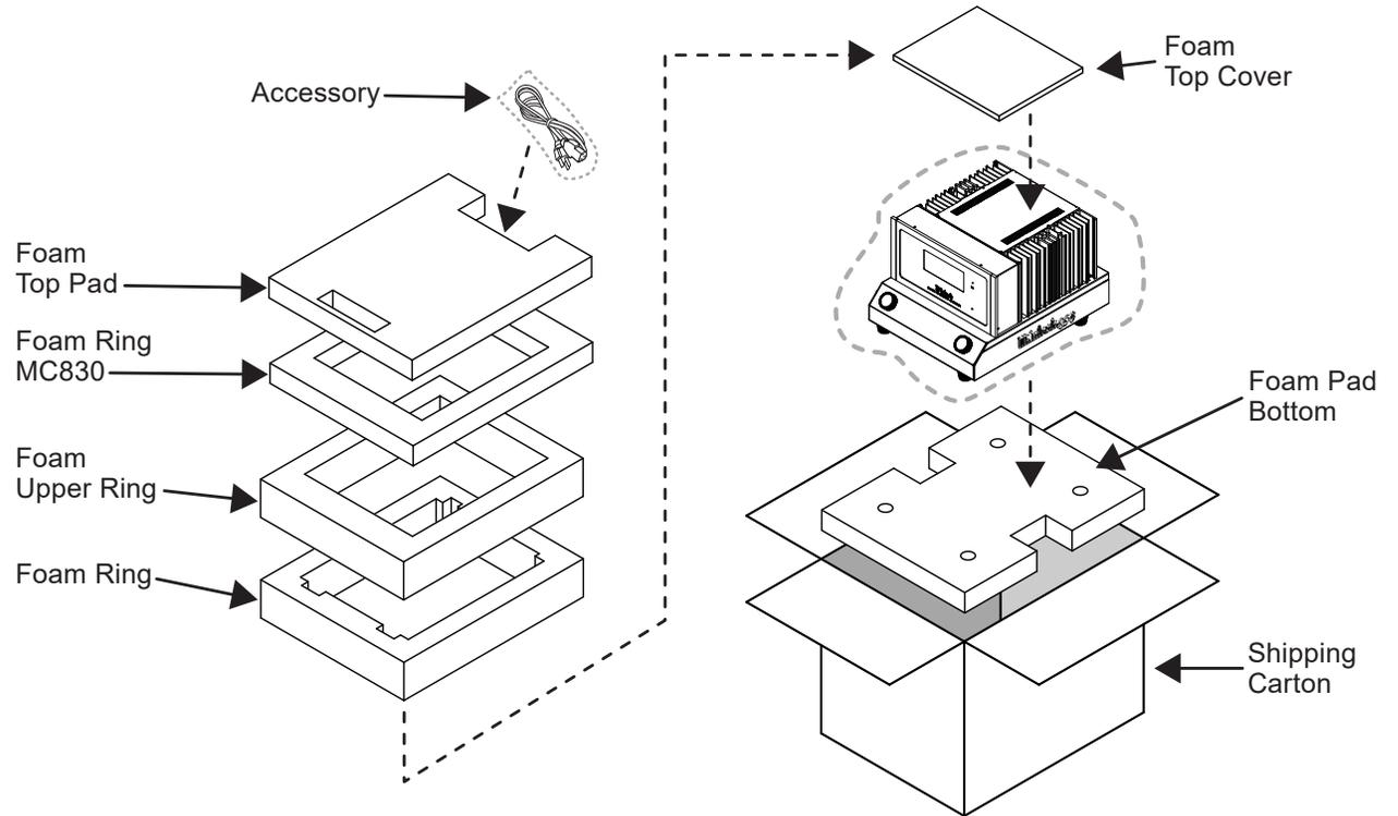
Figure 12– Re-packing diagram
