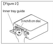
• Place 3 inch/8 cm discs in the inner tray guide without using an adapter.
