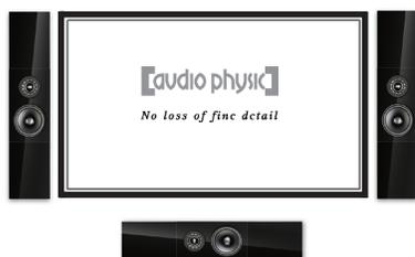
Attach the CLASSIC On-Wall loudspeaker below the television so that the tweeter is on the left-hand side.
